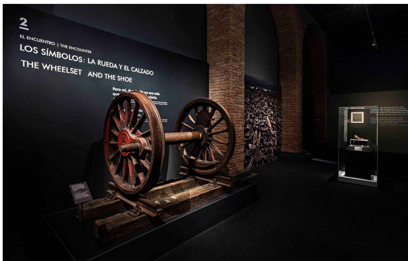
▲ Wheel set from steam locomotive.
